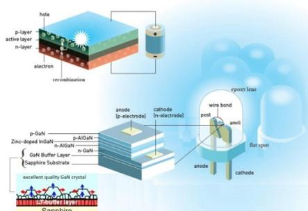
Figure 1 shows the structure of a modern LED. In the inset of the same Figure, the LT-buffer which enabled the growth of the GaN pure crystal is also shown. (Li et al 1993).
